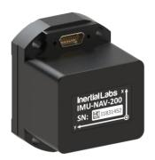
The Inertial Labs IMU-NAV-200 is a breakthrough, fully integrated inertial solution that combines the latest MEMS sensor technologies. Fully calibrated, temperature compensated, mathematically aligned to an orthogonal coordinate system, the IMU contains up to 0.3 deg/hr gyroscopes and less than 0.007 mg bias in-run stability accelerometers with very low noise and high reliability.
