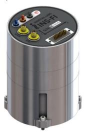
Due to its high-performing FOG IMU, the **INS-FI** can measure GNSS-free Heading (True North) with less than 0.5 deg error, Horizontal & Vertical Positions with approximately 0.1% error of Distance Traveled for land applications, and 5 nautical miles per hour drift for aerospace (Unmanned Aerial Vehicles) applications without GNSS signal.
