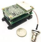
The Inertial Labs **INS-P-OEM** utilizes an advanced single antenna GNSS receiver, barometer, 3-axes each of calibrated in full operational temperature range precision Fluxgate magnetometers, Advanced MEMS Accelerometers and Gyroscopes to provide accurate Position, Velocity, Heading, Pitch and Roll of the device under measure. The **INS-P-OEM** contains Inertial Labs new on-board sensors fusion filter, state of the art navigation and guidance algorithms, and calibration software.
