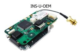
The Inertial Labs **INS-U** utilizes advanced single antenna multi constellation (GPS, GLONASS, GALILEO, QZSS and BEIDOU GNSS) receiver; two Honeywell TruStability® Board Mount Pressure Sensors; a miniature gyro-compensated Fluxgate compass; 3-axes each of calibrated in full operational temperature range Advanced MEMS Accelerometers and Gyroscopes to provide accurate Position, Velocity, Heading, Pitch and Roll of the device under measure.
