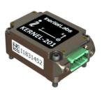
The Inertial Labs KERNEL-201 is a breakthrough, fully integrated inertial solution that combines the latest MEMS sensor technologies. Fully calibrated, temperature compensated, mathematically aligned to an orthogonal coordinate system, the IMU contains up to 0.7 deg/hr Bias inrun stability gyroscopes and 0.005 mg Bias in-run stability accelerometers with up to  $\pm 40$  g dynamic range, very low noise and high reliability.
