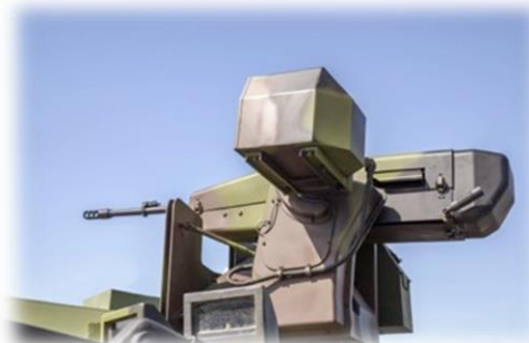
Remote Weapon Stations, EOS stabilization
