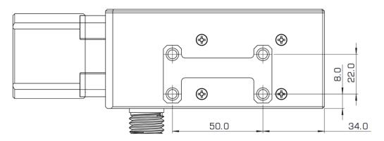
All four mounting holes are threaded M6 x 7mm
