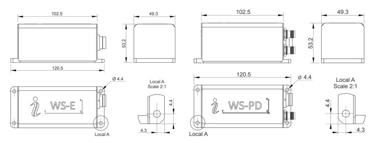
Inertial Labs IP67 sealed Wave Sensors (WS-E, WS-PD) can be easily integrated into existing systems using the following bracket.
