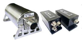
The Inertial Labs **Wave Sensors (WS)** Units utilizes solid state 3-axes each of precision accelerometers, magnetometers, gyroscopes and barometric sensors to provide accurate Wave Characteristics as well as Heave, Sway, Surge, Pitch and Roll of the device under measure.
