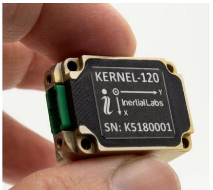
The **Inertial Labs KERNEL-110** and **KERNEL-120** models are the breakthrough, fully integrated inertial solutions that combines the latest MEMS sensor technologies. **KERNEL-120** model utilizes two types of accelerometers: with  $\pm 40\text{g}$  and  $\pm 90\text{g}$  measurement ranges.
