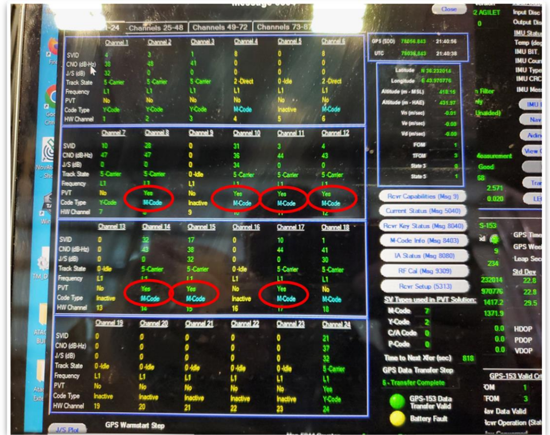
Military GPS User Equipment (MGUE) Inc 1 receiver using 7 M-Code satellites in CENTCOM
