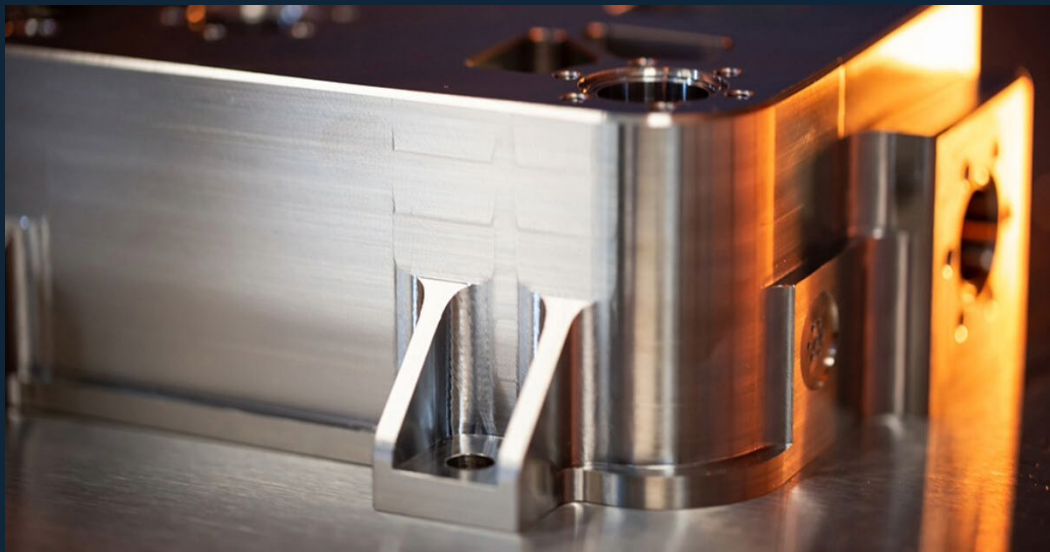
Physics package for atomic gyroscope. Courtesy of Vector Atomic
