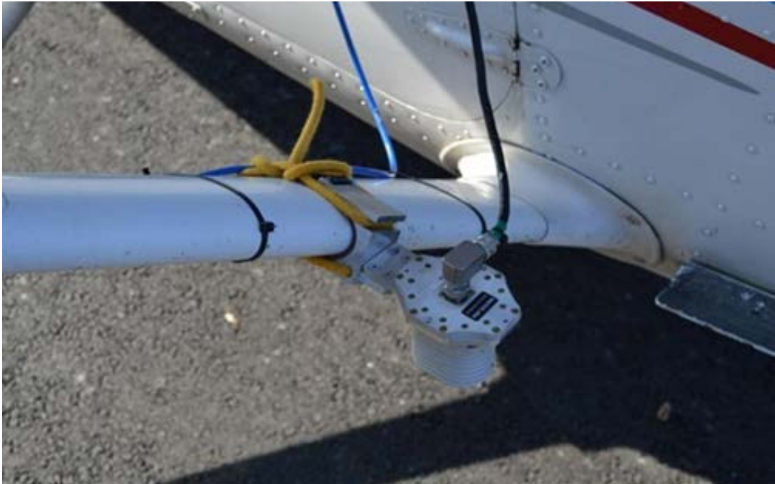
Figure 3.3. Mounting of Sensor Module on the Wing Strut
